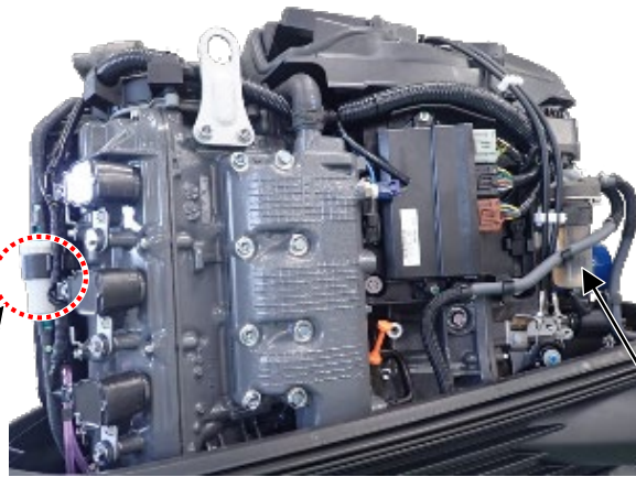
High pressure fuel filter (Passing Particle Diameter: 25 \mu )
